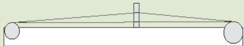
Rigid heddle loom without front and back beams; before weaving
