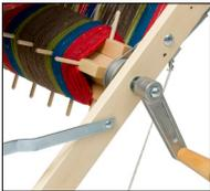
**The Sectional Beam** increases the beam is 12" in circumference and has two-inch sections. It can be added to the existing beam by simply screwing it onto
