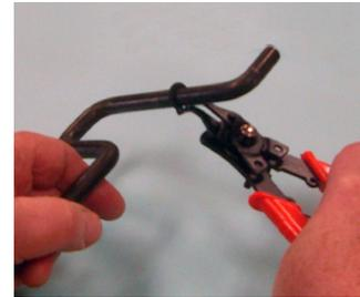
E-CLIP SLIDING ONTO CRANK
