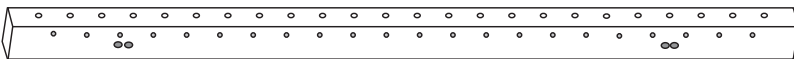
FIGURE E - SECTIONAL BEAM LEAF WITH HOLES FOR CORDS; ONE LEAF PER SECTIONAL BEAM KIT
