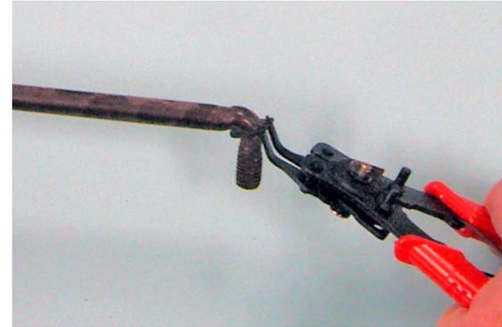
E-CLIP SLIDING ON TO METAL TREADLE SUPPORT BAR
