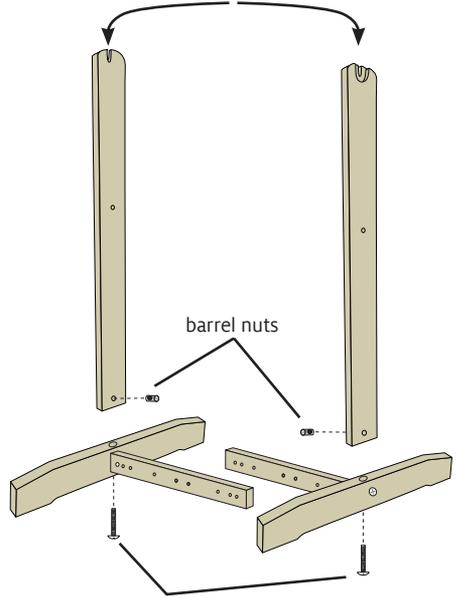
1/4-20 x 3-1/2" Phillips truss head machine screws
